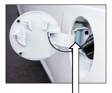
3. Use a ruler to measure the distance from the spring to the edge of the door hinge, as shown. If the distance measured is less than 1.1" (27.9 mm), proceed to the next step. If the distance is greater than 1.1" (27.9mm), no further action is required.
