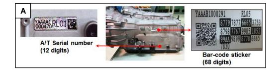
After Transmission Exchange: use GDS/KDS Auto Input Mode. **NOTE:** if internet access is not available, enter in Manual Mode. If you cannot access the internet, record the bar code data (oil pressure characteristics) on the automatic transmission case, and then input it manually on GDS/KDS. Additionally, make sure to perform the TCM adaptive values relearn procedure, using GDS/KDS.
