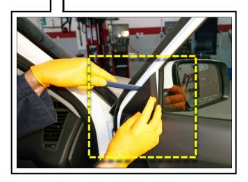
Carefully remove the blanking cover from the mounting location under the door grip, and remove one (1) door panel mounting screw (B).
