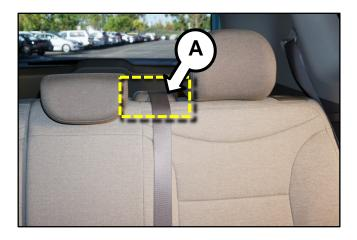
2. Remove the center seat belt guide cover (B) using a trim removal tool, as shown.
