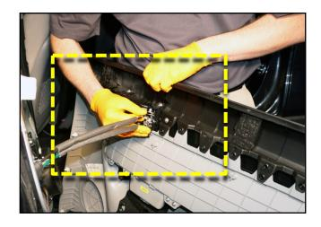
13. Remove four (4) screws securing the door interior door handle cage to the door panel.
