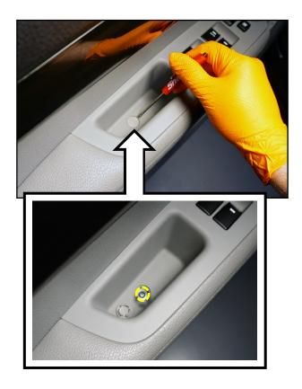
9. Carefully remove the blanking cover from the outermost mounting location and remove one (1) door panel mounting screw.
