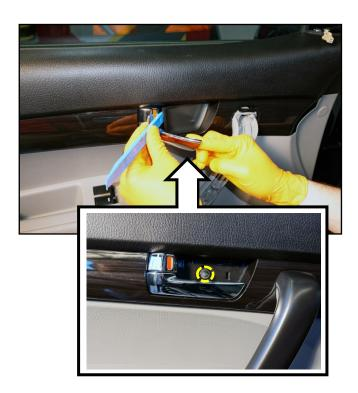
7. Carefully remove the blanking cover from the innermost mounting location and remove one (1) door panel mounting screw.
