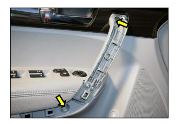
6. Remove trim cover from inside door handle area and remove one (1) door panel mounting screw.
