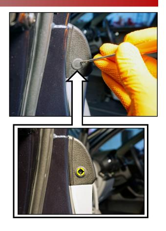
10. Use trim panel remover to dislodge the bottom edge of the door panel and remove the door panel by applying gentle outward pulling force.
