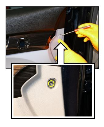
8. Carefully remove the blanking cover from inside the door grip area and remove one (1) door panel mounting screw.
