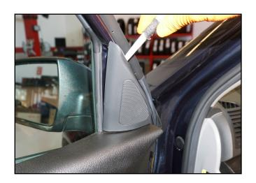
Use a non-marring trim panel remover to disconnect the speaker connector, as shown.
