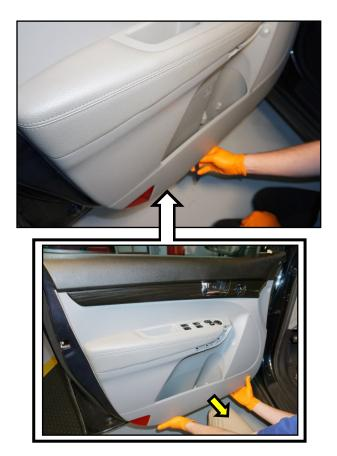
11. Carefully disconnect all connectors from the back of the door panel.
