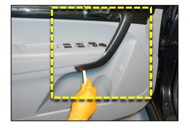
5. Remove two (2) door panel mounting screws from the door grip area.
