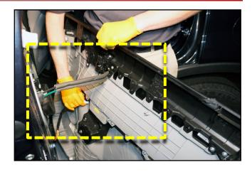
12. Disconnect the door latch mechanism from the interior door handle.
