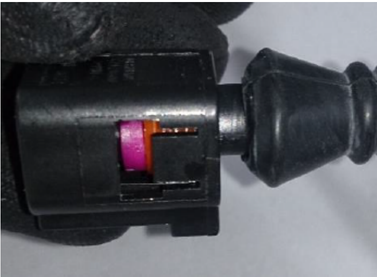
9. Mount the protective boot on the connector.
