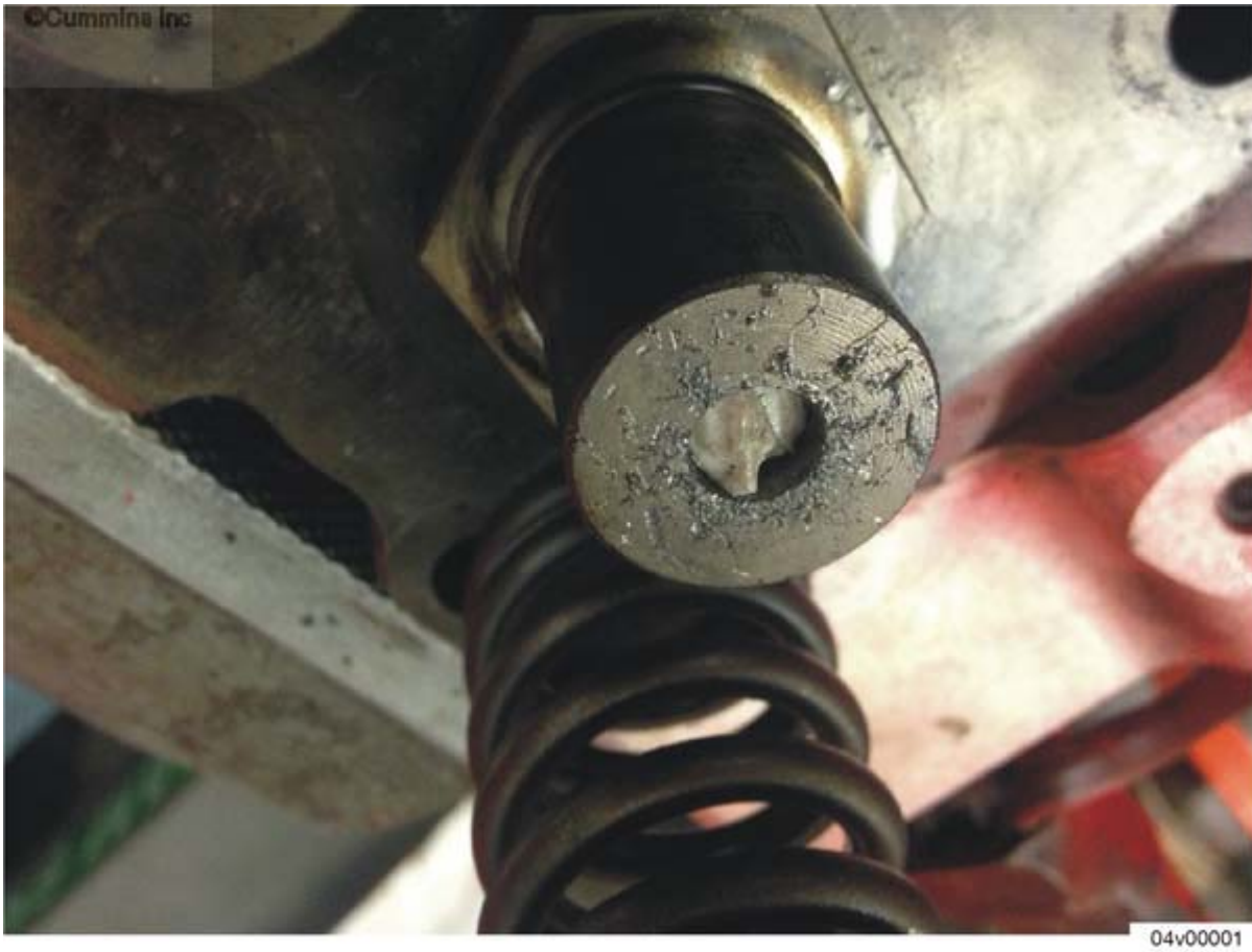
Figure 1: Fractured Fuel Pump Ceramic Pumping Plunger
