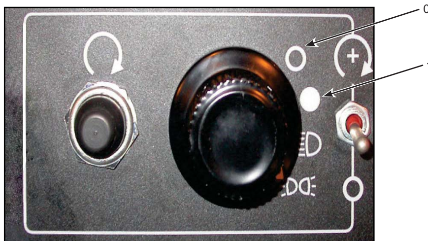
Figure 1 - Master Control Switch
