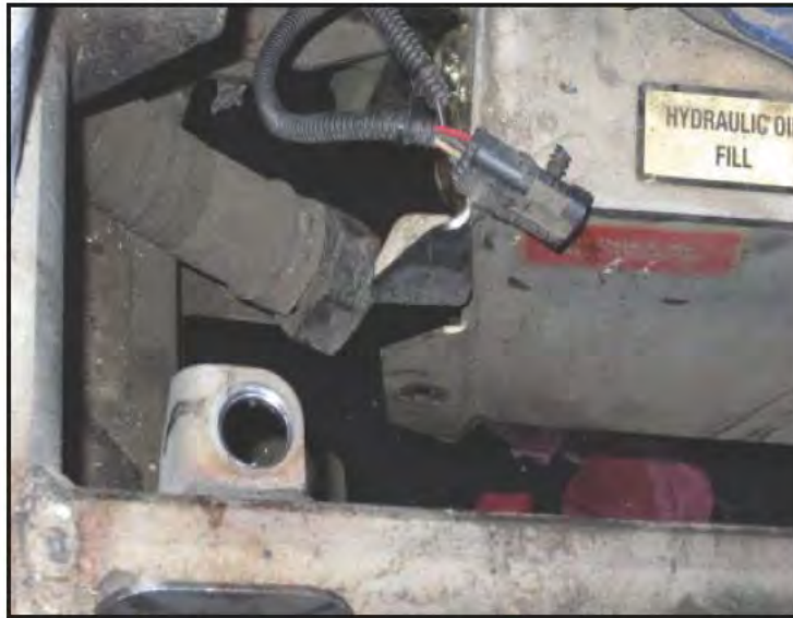
Figure 12 - Move the Tank Away from Brackets
