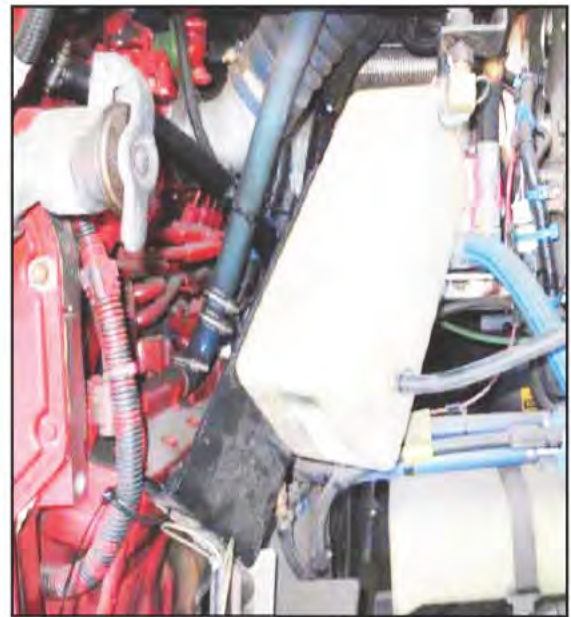
Figure 6 - Move Surge Tank Forward
