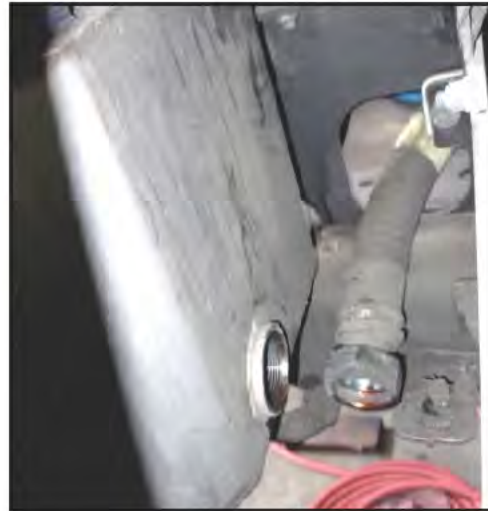
Figure 8 - Disconnect Hose and Remove Fitting
