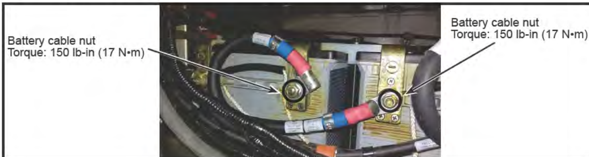
Figure 9 - Torque Values for Battery Connections
