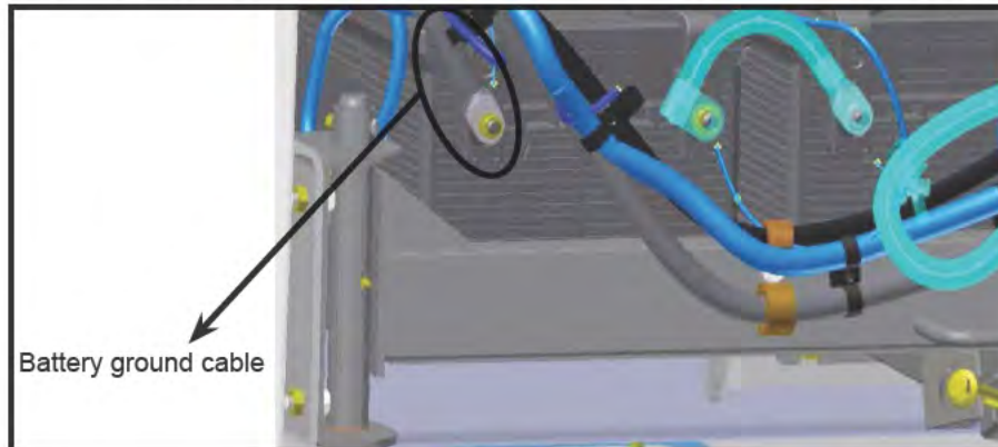
Figure 3 - Location of Battery Ground Cable
