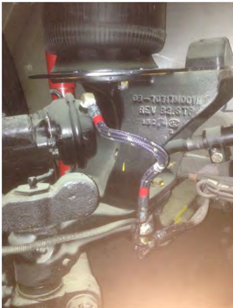
Figure 3: 16" Replacement brake line (Curbside shown)
