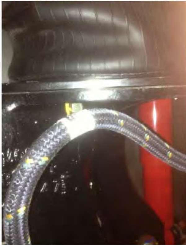
Figure 1: Airbag mounting surface. (Roadside shown)
