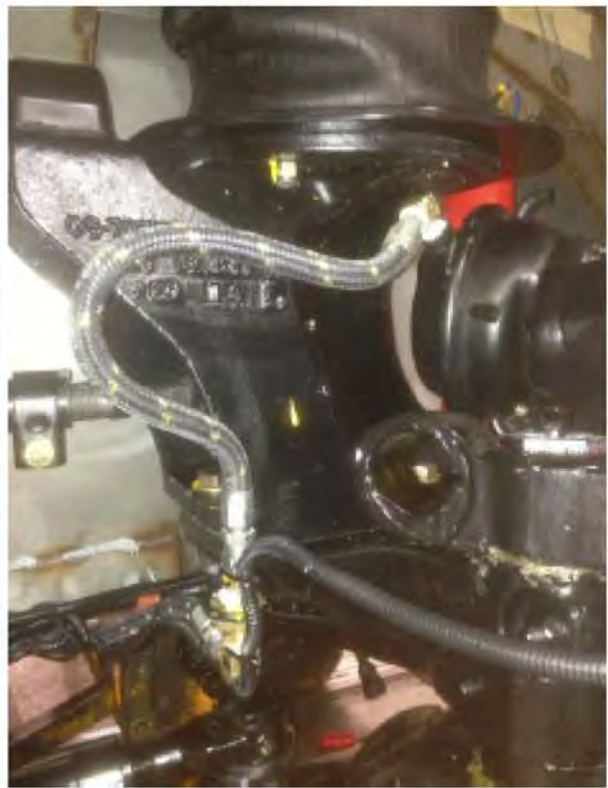
Figure 2: Suspension tower wall. (Roadside shown)
