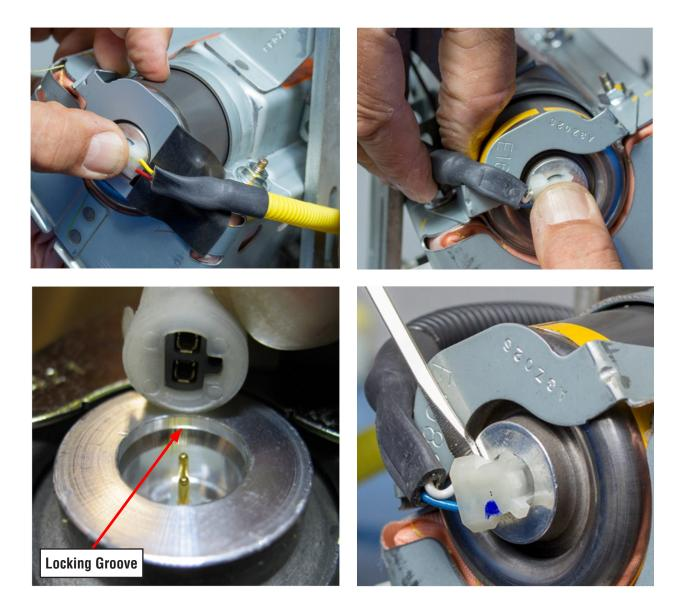
**STEP 12-** Refit the ends of the harness corrugated tubes to the retaining grooves of the mounting bracket as shown to complete the airbag module reassembly.
