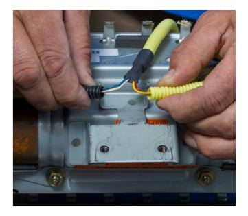
STEP 3- CAREFULLY cut the yellow harness cover (approximately 1 1/2 inches) enough to expose the 2 yellow and red wires inside and provide enough room to install the Electro-Tap (shorting) connector using a scissor or wire cutter (no knives or razors).
