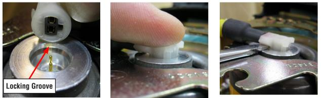
**STEP 12-** Reinstall the airbag assembly into the vehicle in reverse order of disassembly. Before installing the glove box assembly, reconnect the negative battery cable. Turn the ignition key "ON" and confirm the AIRBAG warning light comes on then cycles off properly. Once proper warning light operation is confirmed, reinstall the glove box assembly to complete the procedure.
