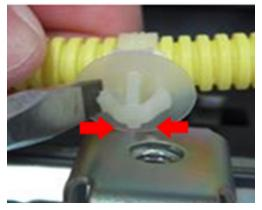
**STEP 3- CAREFULLY** cut the yellow harness cover enough (approximately 2 inches) to expose the 2 red or yellow wires inside and provide enough room to install the Electro-Tap (shorting) connector using a wire cutter or scissor (no knives or razors). **TAKE YOUR TIME AND BE CAREFUL TO NOT CUT THE 2 WIRES!**
