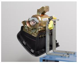
**STEP 2-** Peel the Sponge Tape and remove the harness clip from the retainer bracket by pushing the tangs inward with a flat-blade screwdriver as shown below. Always remove any Sponge Tape adhesive residue from the airbag mounting bracket using mild solvent on a clean shop cloth. **CAUTION:** Never use any silicone-based products for this purpose.
