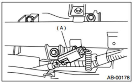
• Remove the 3 retaining bolts and **CAREFULLY** remove the airbag module from the vehicle and place it on a clean cloth to protect the dash trim outer surface portion from damage.
