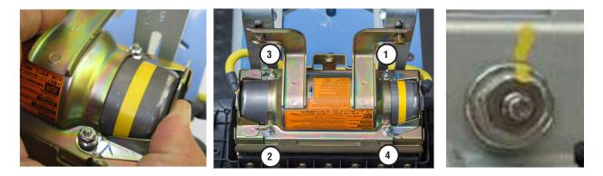
**STEP 11-** The new inflator wiring harness has a "long side" and a "short side" with round 2-pin connectors on both ends. The short side with red wires will connect to the end of the inflator with the round wiring harness connector boss, yellow tape and removable stopper plate. **VERY IMPORTANT:** When connecting the new harness to the inflator, both sides of the harness **MUST be routed toward the module's mounting brackets as shown in the photos below.**
