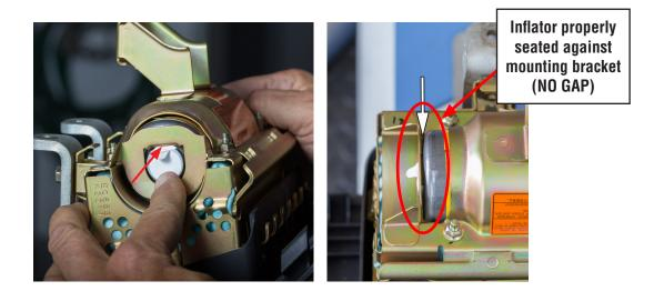
**STEP 10-** As shown below, install but do not fully tighten 2 of the NEW self-locking nuts while holding the stopper plate tight against the inflator. Remove the nuts still installed on the mounting bracket and replace them with 2 **NEW** self-locking nuts. Once all 4 **NEW** nuts are in place, torque to 31 - 38 inch pounds in the sequence shown below. Use a marker to mark the nuts after torquing indicating they have been fully tightened.
