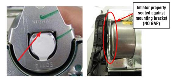
**STEP 10-** As shown below, install but **do not fully tighten** 2 of the NEW self-locking nuts while holding the stopper plate tight against the inflator. Remove the nuts still installed on the mounting bracket and replace them with 2 **NEW** self-locking nuts. Once all 4 **NEW** nuts are in place, **torque to 31 - 38 inch pounds in the sequence shown below**. Use a marker to mark the nuts after torquing to indicate they have been fully tightened.
