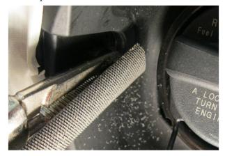
• Using the fine flat file and very short strokes, restore the radius (curvature) to the end of the lock pin by **CAREFULLY** removing a small amount of material from the outside perimeter (face) of the lock pin. Use the detail illustration below as further reference.
