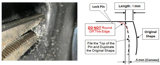
• Use a small piece of a Scotchbrite surface conditioning pad to remove any remaining roughness or burrs left on the lock pin to leave a smooth finish as shown below.
