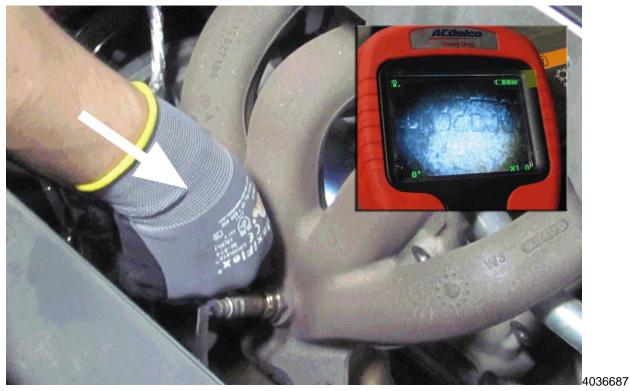
3. Route the borescope under the exhaust manifold as shown in the photograph to gain access to the engine block.
