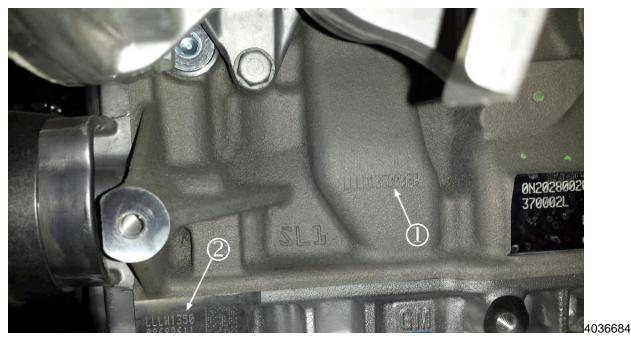
**Note:** A borescope is required to view the engine block number (1) and engine block bed plate (2) numbers.
