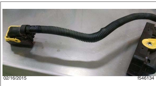
Fig. 7, Harness Wrapped with Convolute
