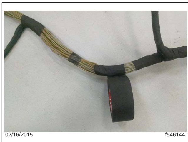
Fig. 14, Wrapping the Harness with Fiber Tape
