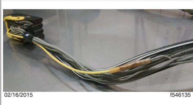
Fig. 5, Splicing the Wires
