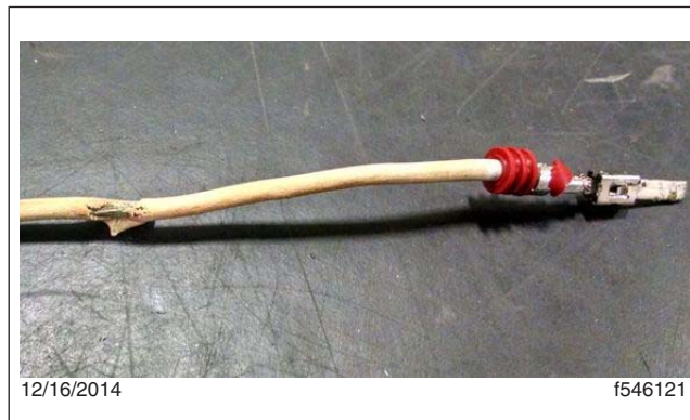
Fig. 2, Insulation Discoloration, Major
