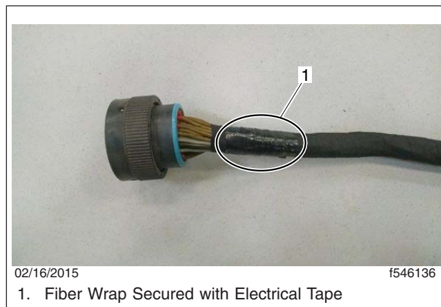
Fig. 15, Fiber Wrap Secured with Electrical Tape
