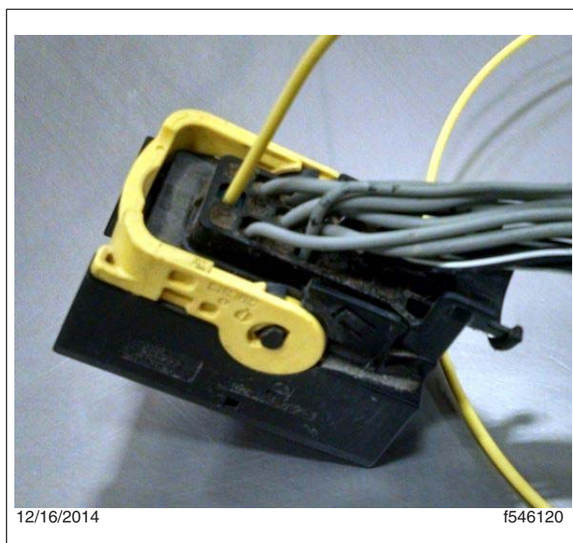
Fig. 3, Terminal Inserted Into the Connector
