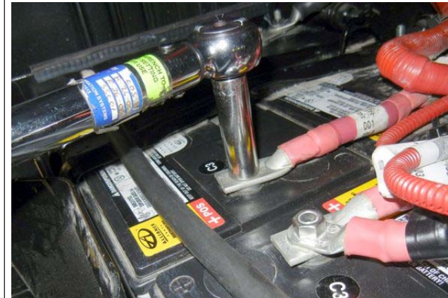
Fig. 11, Check the battery connections for looseness and corrosion. Check the torque on the connections.
