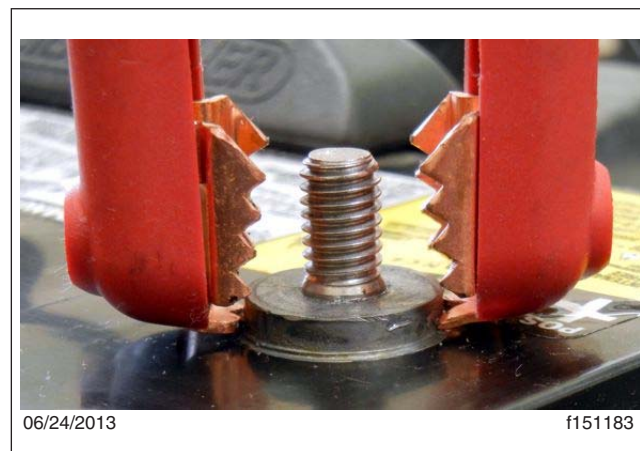
Fig. 3, The lead base of the post is the best place to clip.
