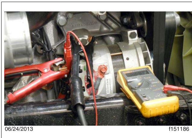
Fig. 5, Alternator Positive Cable Check
