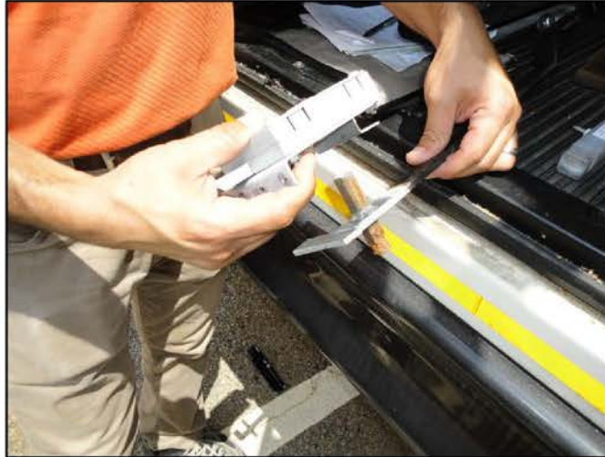
Figure 9, Removing the Locking Mechanism
