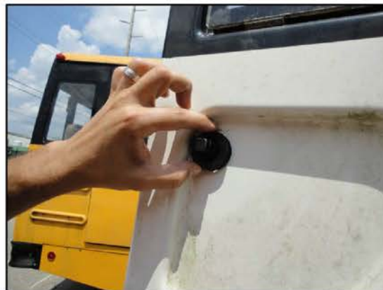
Figure 10, Installing the New Washer
