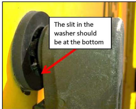
Figure 5, Position of Slit in Washer
