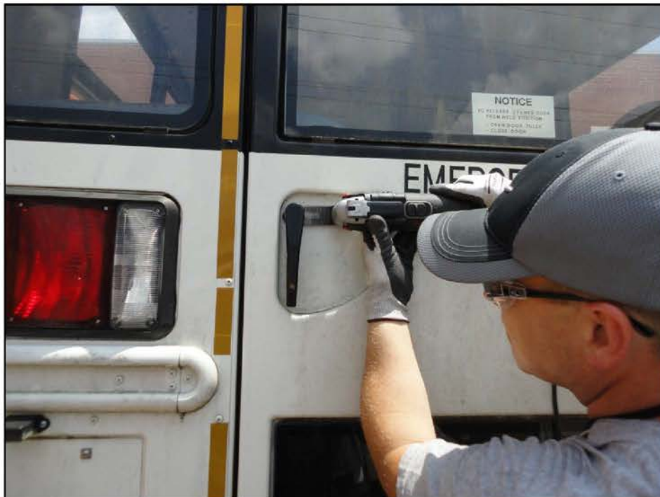
Figure 6, Cutting Off the Stem and Exterior Door Handle
