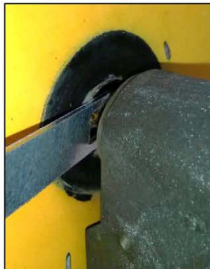
Figure 3, Using the Go/No Go Gauge
