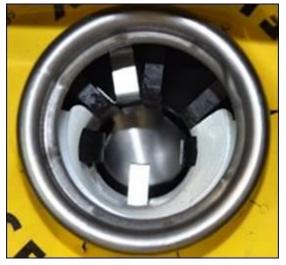
**Figure 1.** Misfueling guard installed in the filler neck.
