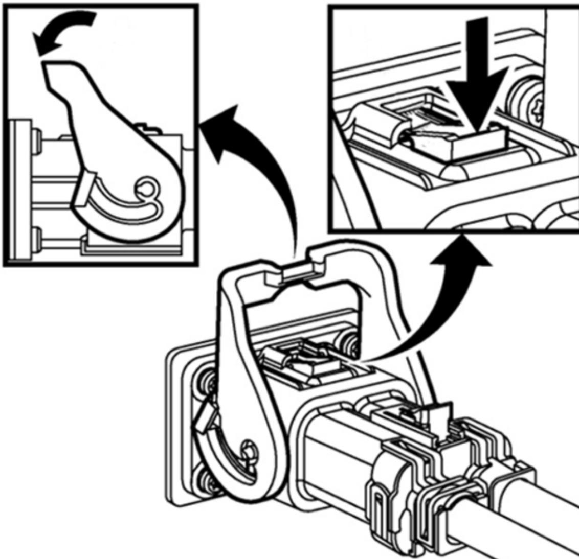
2. Depress the connector lock. Keep the lock depressed and rotate the lever forward to the pre-stage position. There will be an audible click sound when the connector lock disengages.
