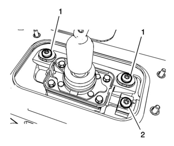
**10.6.** Tighten the shift control mounting bolts (1) to 30 N•m (22 lb ft).
