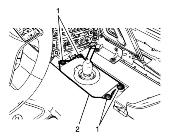
$\textbf{12.} \ \ \textbf{Install the lower transmission control closeout boot (2)}.$
