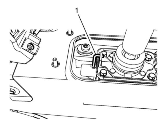
11. Lift to release the shift control neutral lock pin (1).
