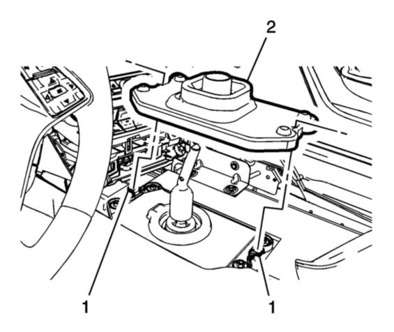
**2.** Remove the upper closeout boot (2) from the transmission control assembly.
