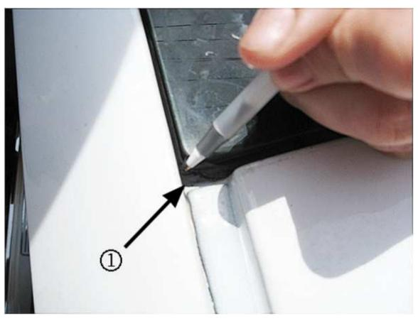
4. Also inspect the forward-most edge of the ditch, assuring any gaps in the factory sealer are filled. Inspect and seal all the way to and below the rubber windshield lace (1).
