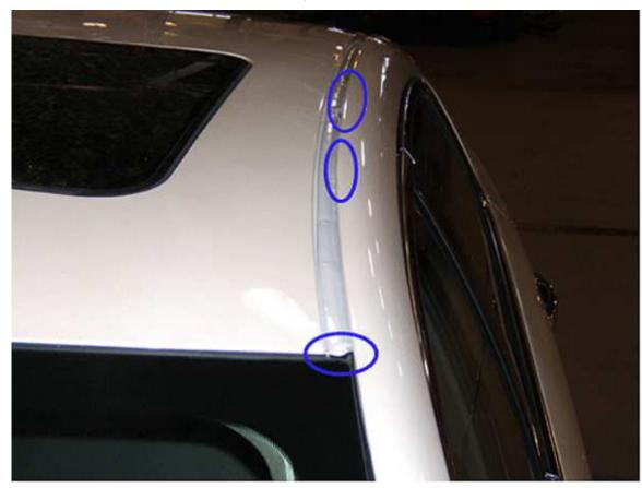
This condition may occur due to incomplete sealing within the roof to windshield header, A-pillar and/or B-pillar seams.
