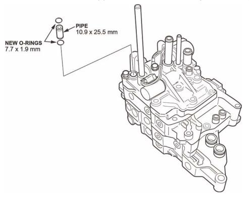
8. Install the new lower valve body and the bolts. Tighten them in a crisscross pattern in at least two steps.
