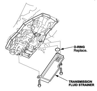
7. Inspect and clean the inlet opening of the transmission fluid as needed. Replace it if clogged or damaged.
