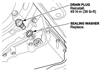
4. Reinstall the drain plug with a new sealing washer.
