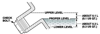
17. Reinstall the check bolt with a new sealing washer.
