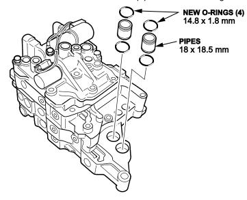
2. Transfer the 10.9 mm x 18.6 mm pipes with new O-rings onto the new lower valve body.
