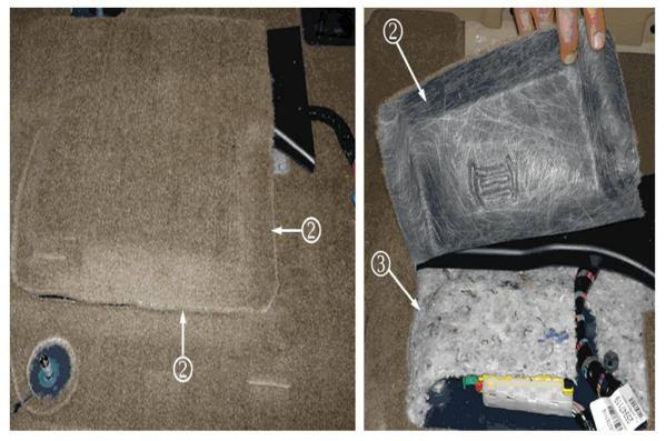
**Note:** Carpet and cutout flap (2) shown with the driver's seat removed from the vehicle for illustration purposes only. Seat removal is NOT required to gain access to the acoustical pad (3).
