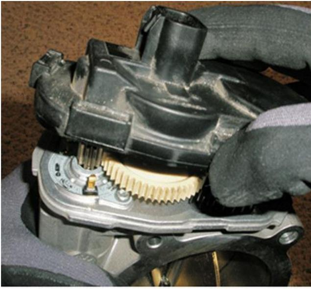
18. Position and install the TP sensor cover to the throttle body. Hold the TP sensor cover in position. If necessary for ease of the clip installation, secure a rubber band around the throttle body and TP sensor cover.
