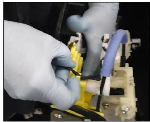
10. Unclip the plastic housing (F) from the door latch assembly (G) using a flat head screwdriver.
