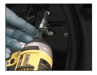
8. Remove the door module panel assembly (E) bolts and disconnect the door harness connector.
