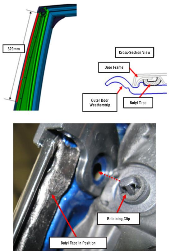
After the butyl tape is applied, refit the door frame weatherstrip and make sure the retaining clip "clips" back into the hole as shown to properly secure and position it. Work the weatherstrip onto the butyl tape with your thumbs making sure it is smooth and any bumps or high spots have been worked out.
