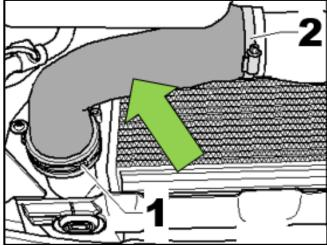
Reinstall the air guide hose <arrow>, and fasten the clamps <1 and 2>.
