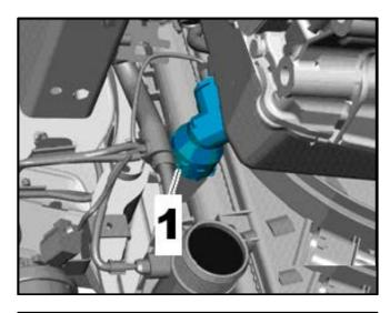
• Reconnect the lower coolant hose <1> to the radiator.
