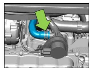
Reinstall the lower coolant hose onto the After-Run Coolant Pump V51 <arrow> and fasten the clamp.
