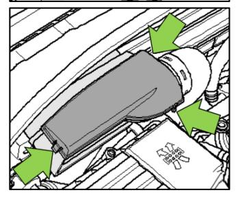
Reinstall the air duct cover and refasten the side clips <arrows>.
