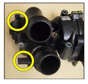
• Reconnect both electrical connectors <circles> on the coolant pump housing.
