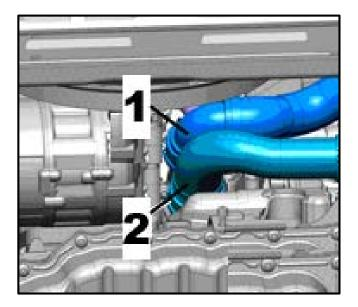
Remove the coolant hoses <1 and 2> and allow the coolant to drain.
