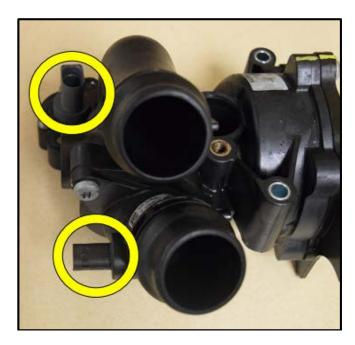
Disconnect both electrical connectors <circles> from the coolant pump housing.
