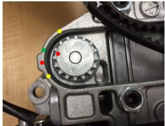
Figure 8. Placing a green dot in between the two yellow dots and turning the gear (red dot) to match the green dot on the housing.
