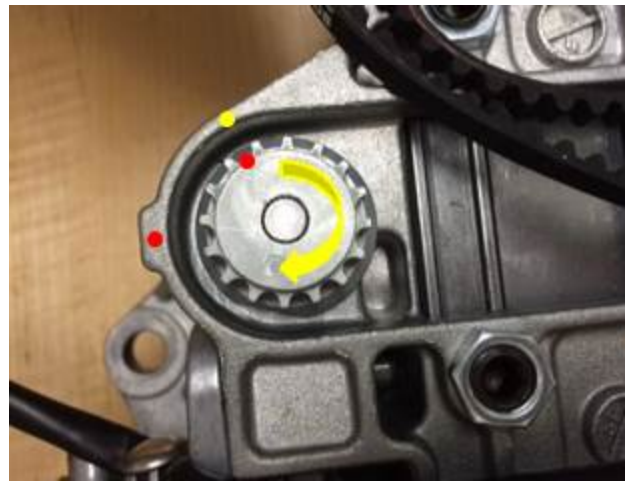
Figure 6. Marking the location with the greatest resistance in the clockwise direction.
