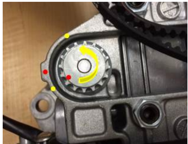
Figure 7. Marking the location with the greatest resistance in the counter-clockwise direction.
