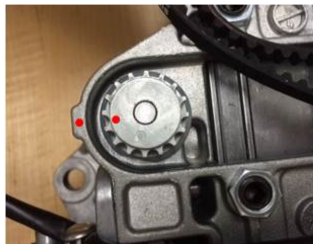
Figure 5. Marking original gear location.
