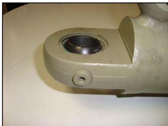
Figure 1: Pivoting point of hydraulic cylinder fitted with a plug instead of a grease nipple
