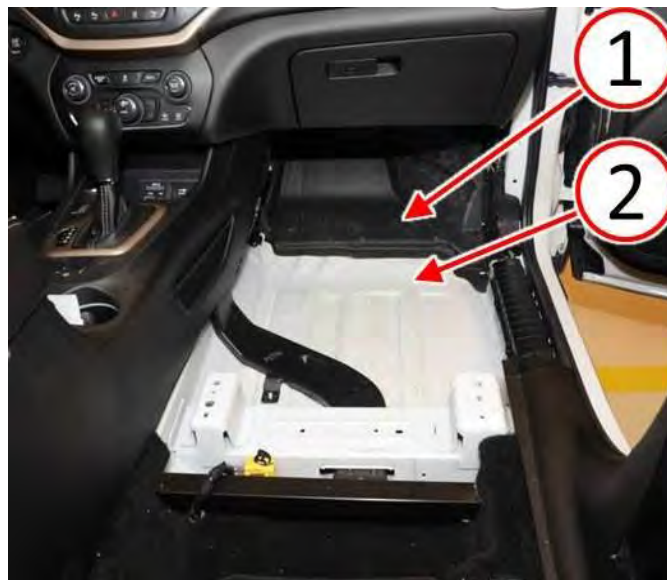
Fig. 12 Inspect For Water Leak
