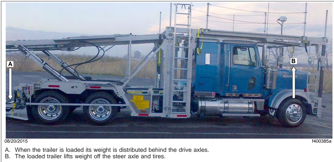
Fig. 2, The Effect of Adding Weight on the Car Hauler
