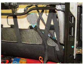
26. Secure the harness in position underneath the cushion cover straps, as shown above.
