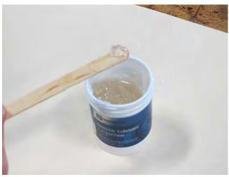
16. Before reinstalling the seat, apply dielectric lubricant (clear gel), GM P/N 12377900 (in Canada, use P/N 10953529), completely across the terminals on both sides of the seat and main body harness connectors.
