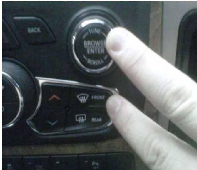
Fig. 2 Take Vehicle Out of Ship Mode
