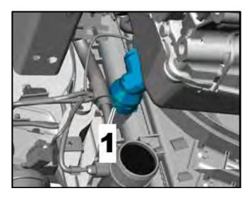
Reconnect the lower coolant hose <1> to the radiator.
