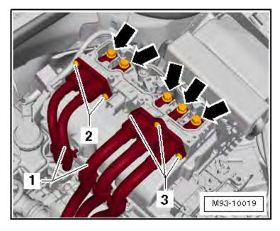
Tightening Specifications, High Voltage Contacts
