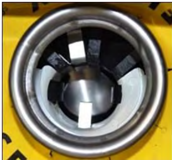
Figure 1. Misfueling guard installed in the filler neck.
