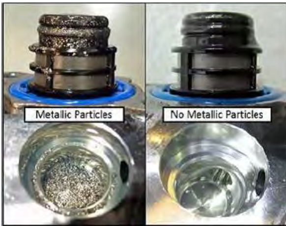
Figure 3. N290 Fuel Metering Valve and Valve Bore
