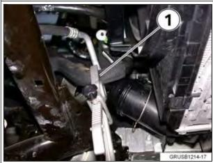
Clamp off the outflow hose (1) on the cooler with special tool 81 64 2 184 117 (SI <u>B04 07 11</u>). The outflow hose is the softer (rubber) of the two cooling lines on the heat exchanger.
