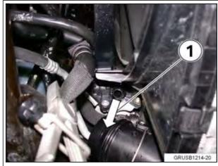
If any coolant starts leaking out of the transmission heat exchanger (1), the internal thermostat is jammed and the heat exchanger will need to be replaced. Follow Repair Instruction RA 17 22 010, "Removing and installing/replacing transmission oil cooler for automatic transmission (N20, N26, N55)."
