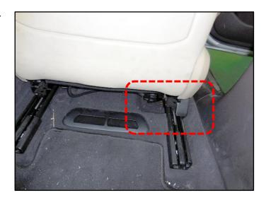
3. To release the locking mechanism, rotate the lever (C) in the direction of the arrow.
