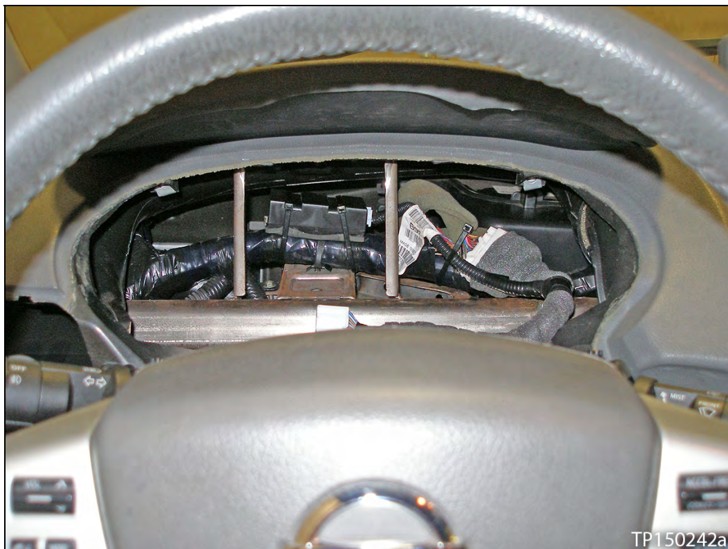
Figure 4: Amp and jumper harness installed
