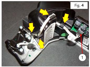
Undo the indicated screws and remove the left hand turn indicator button (B)
