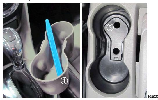
11. Remove the rubber cup holder liner (4) and plastic cup holder access panel (5).
