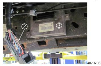
8. Disconnect the chassis wiring harness electrical connector (2) from the fuel pump flow control module (3).
