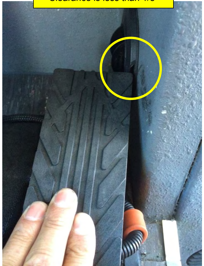
Clearance is less than 1/8 "
