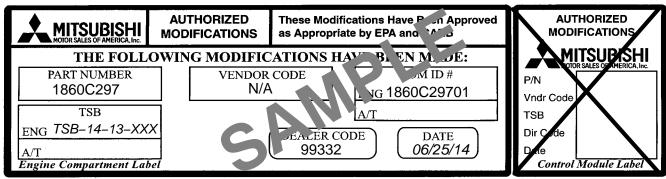
The Control Module Label is NOT used for this reflash. It should be discarded.
