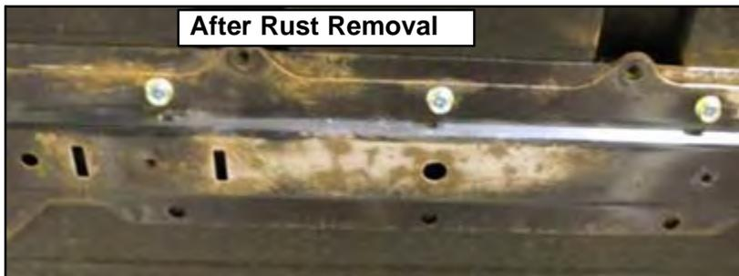
7. Repeat Step 6 for Crossmember B, C, and D and remove rust if required.
