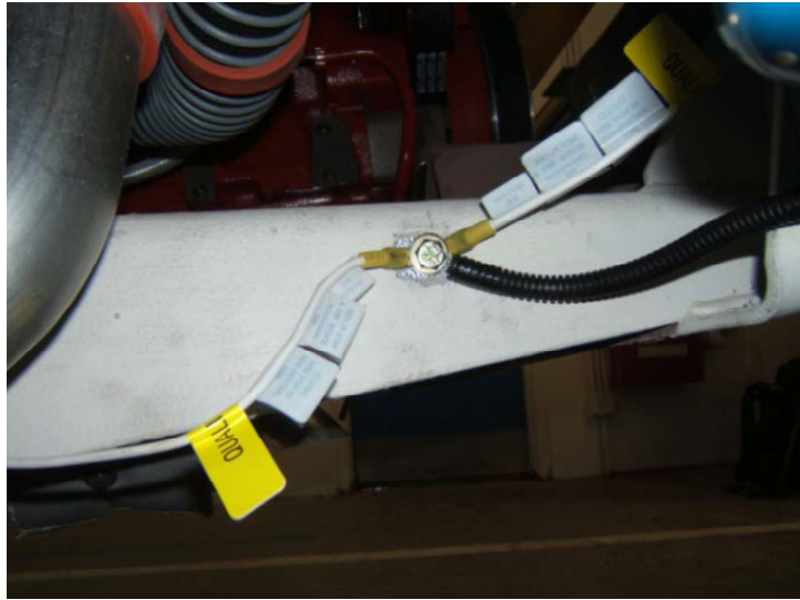
Figure 10: Common Ground Point on Bus Frame
