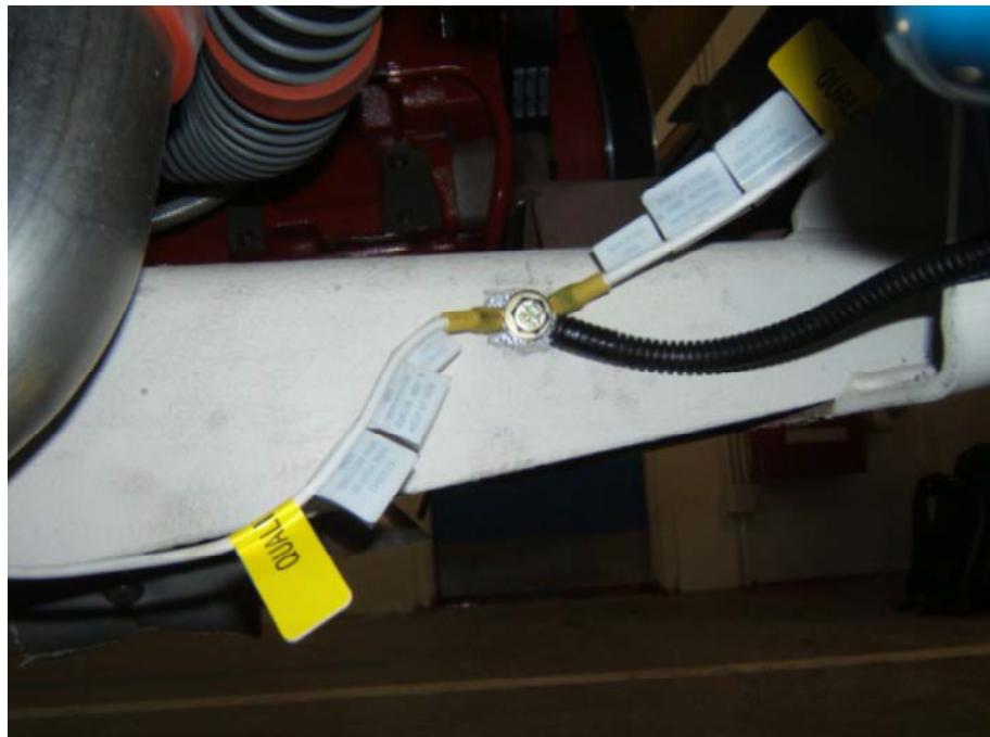
Figure 7: Common Ground Point on Bus Frame
