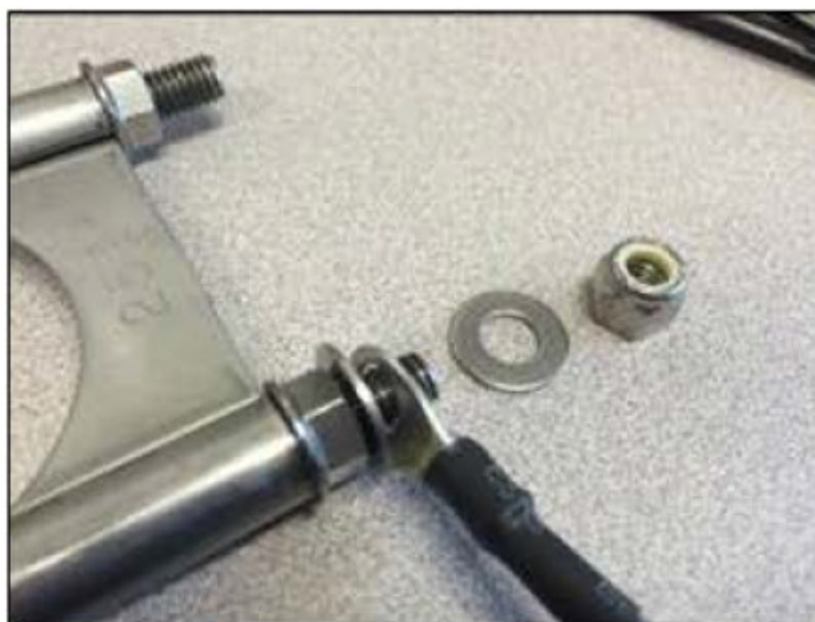
Figure 3: Ground Strap Mounting Hardware Orientation
