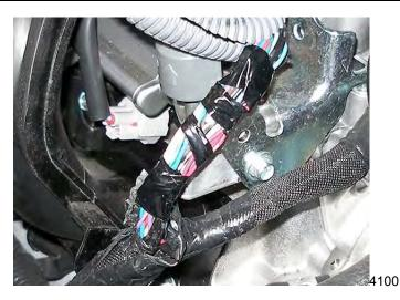
16. Wrap the wires with electrical tape or equivalent.
