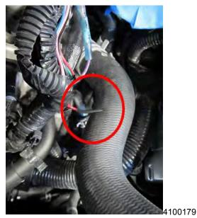
**Note:** Only use heat shrink tube, P/N 12355010, or an equivalent flexible adhesivelined/moisture resistant heat shrink tube to perform the repair in this bulletin.
