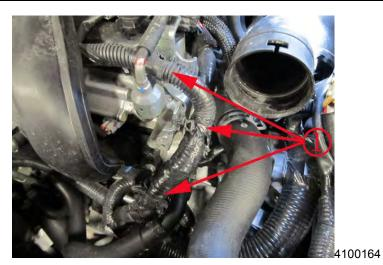
Disengage the three retainers (1) as illustrated above. 5.
