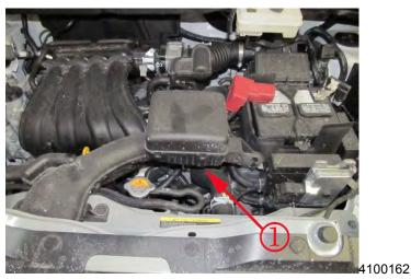
3. Remove the Front Intake Air Duct (1).
