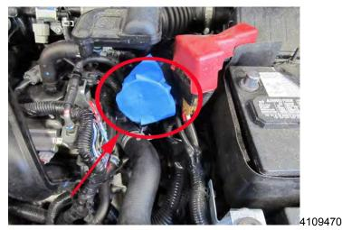
**Note**: This step is to ensure nothing enters into the duct during the procedure. The graphics in subsequent steps do not show the intake being blocked as photos of a properly covered intake were not available. Ensure the intake duct remains covered as in the graphic above.
