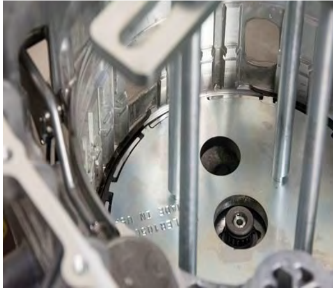
Fig. 11 New Snap Ring Installed
