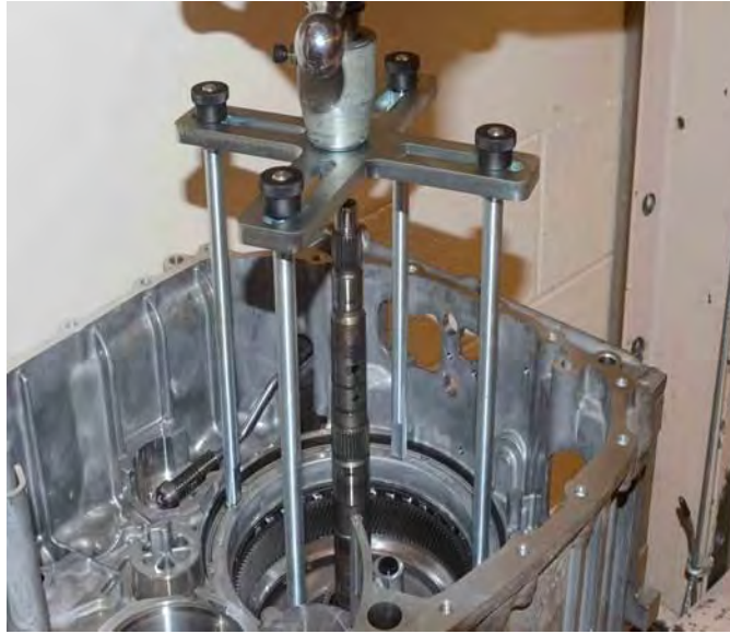
Fig. 8 Pressing Tool Installed
